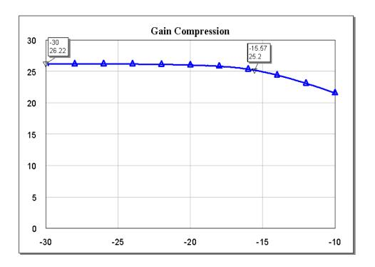
Pout at 1 dB compression = 10 dBm@9 GHz
